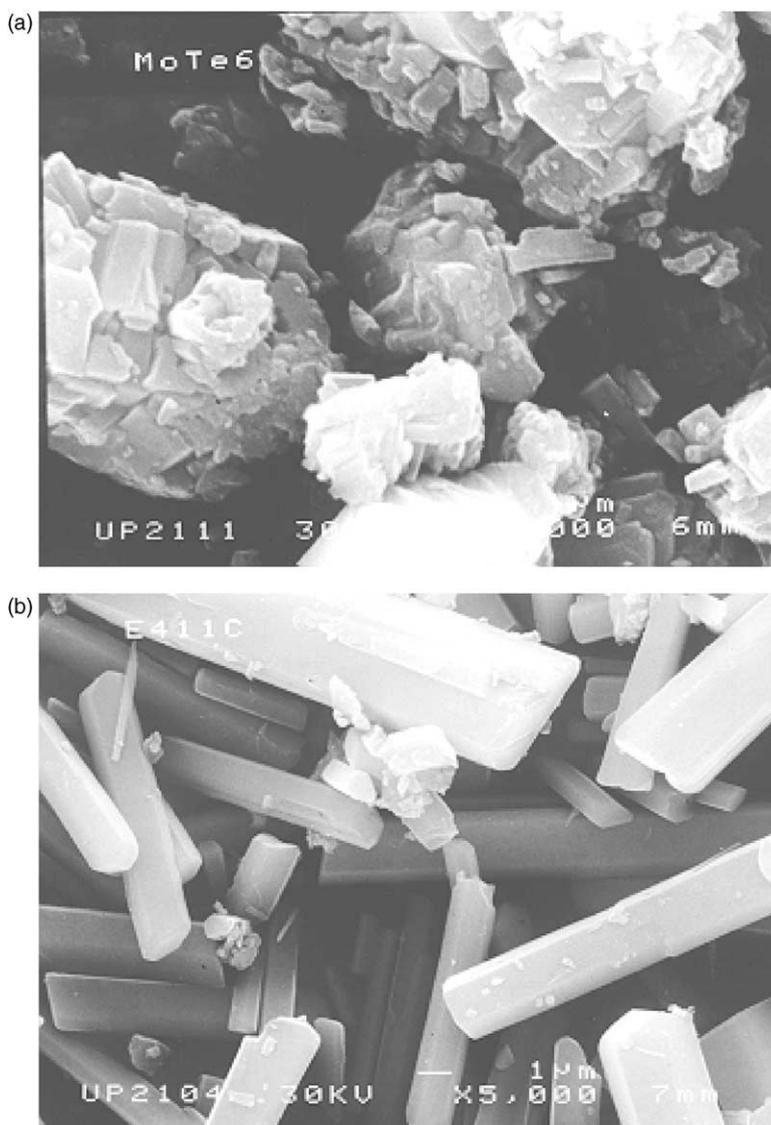
Fig. 4. SEM micrographs of as-synthesised samples: (a) SL; (b) HT.
